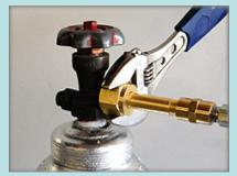
3) After you make sure all the fittings on the CO2 tank are tight, open the valve on the tank. Check for any leakage.
